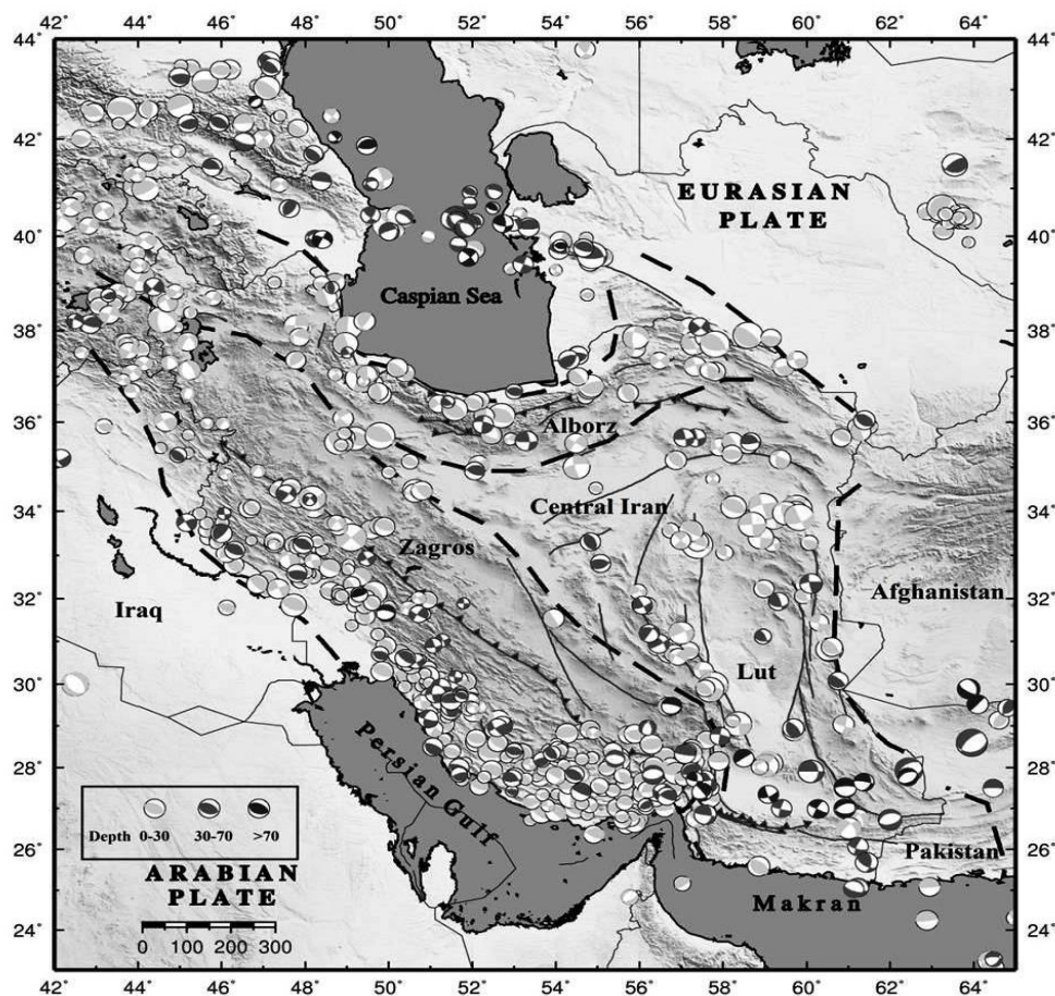
Fig 1. Focal mechanism of the main earthquakes recorded in Iran during the last century. dashed lines: borders of the 3 main tectonic zones of Iran. solid line: major faults (adapted from Shahvar et al., 2013).
